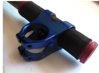
After assembly of the stem and fastening of the bolts please check if the stem is really fixed on the steerer by clamp the front wheel between your legs and try to turn the handlebar.
