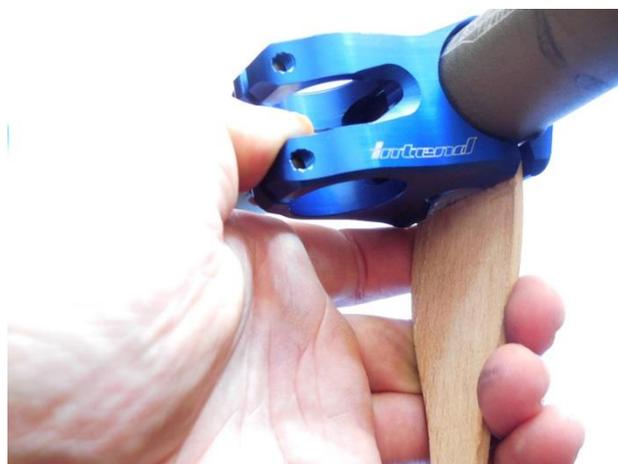
Please Note: if this step is done not carefully, the surface can get some slight scratches. The stem has to be opened wide enough to ensure not to need to much force pushing in the handlebar.
