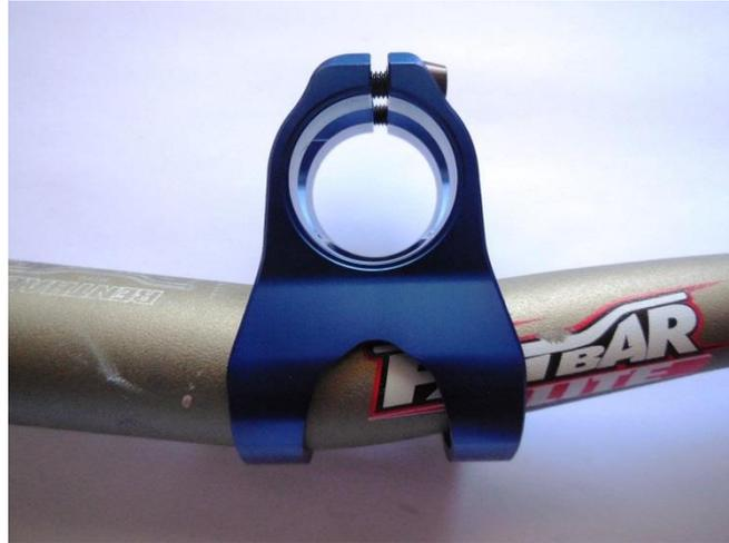
To get the handlebar in the stem the handlebar clamp has to be opened slightly with the included wooden spoon. The easiest way is shown in the pic, look at the chamfer ! (Fase am Holz)! Please note that the wooden spoon should not extend in the handlebardiameter because the handlebar should take place there later.
