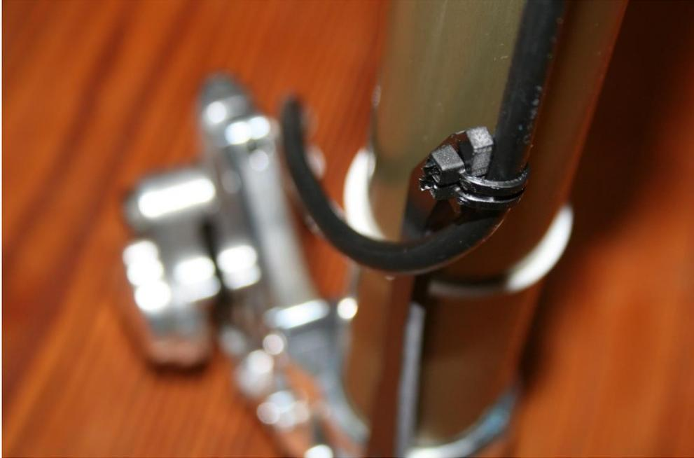
The brake cable has to come from the inside to avoid contact between the cable and the upper leg in case of compression.
