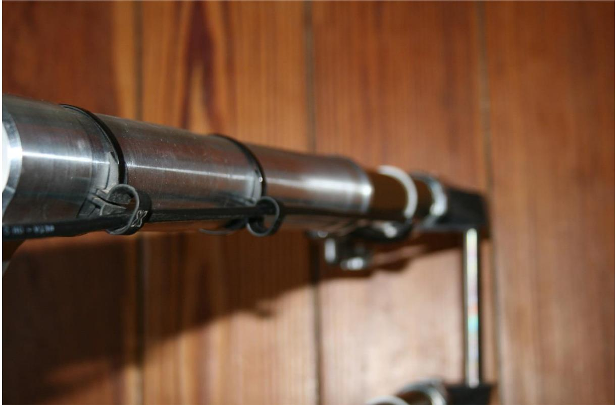
Then install the upper guides as usual. The lower one has to have a minimum distance to the hose arm bigger than the fork stroke to avoid contact in case of compression.
