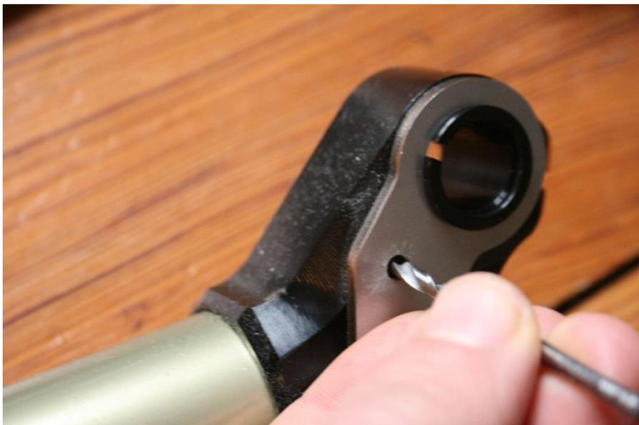
Drill a hole with the delivered 4,2mm drill carefully (only the shown side, the inner side is hollow, the thickness is around 5mm, so you will feel clearly if you are in). Afterwards remove the template and deburr (entgraten) the edges of the drilling hole a little bit with a sharp knife.
