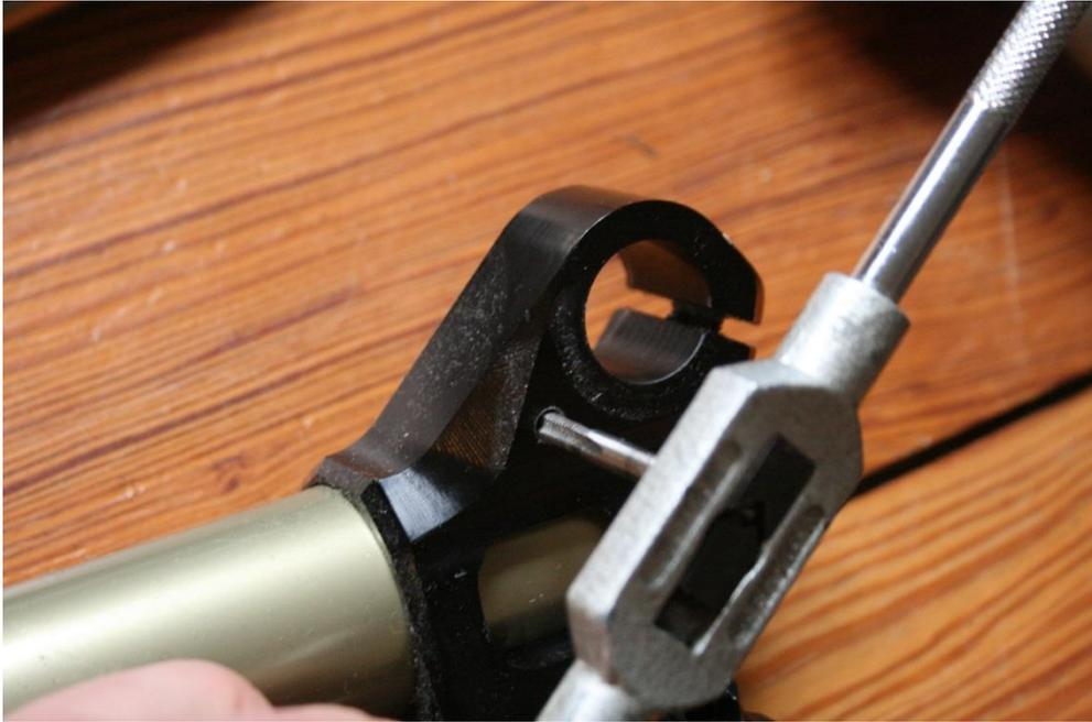
Take the M5 thread cutter. Please make sure that this is aligned 90° to the surface.
