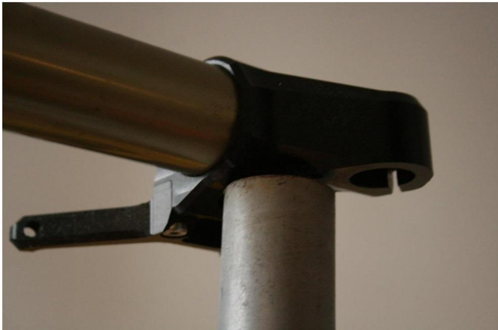
Then take a vacuum cleaner and hold the fork “upside down” to remove all aluminum chips from the inside. It helps if you shake the fork a little bit.
