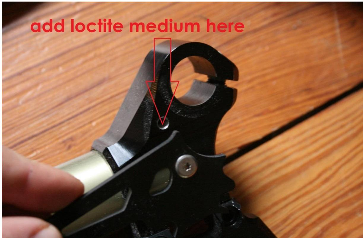
Then mount the hose guide arm with the bolt. TX10 – around 3-4 Nm.
