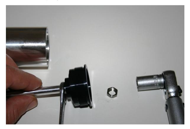
You will find a rubber bottom out ring in the double crown fork, just put this back again in the tube, it is not necessary that this ring has a proper seat, it is only important that it is inside and it will work well!
