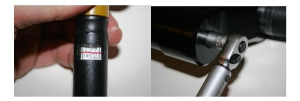
Fasten the hex nut with 10Nm at both sides.
