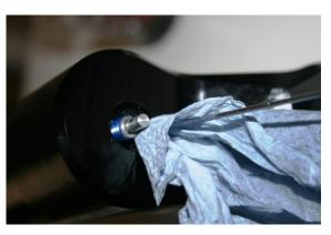
Unscrew the hex nut with a 10mm socket nut. Afterwards pull out the lower tube carefully and release the old oil out of the upper leg. And clean the inside.
