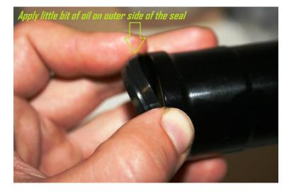
The following step ensures that the seal has a correct seat in the groove.
