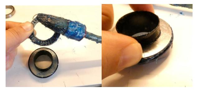
The next step is to place the big o-ring in its groove. The o-ring is a little bit smaller than the groove. Always hold the axial bearing in place(otherwise the o-ring will pop between axial washer and the upper cup) and pull on the o-ring in the groof. I always use the nail of my finger to push it in the groove all around.
