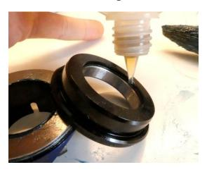
Now you can assemble the both halfes: The inner shell should be in the position like shown and then you can push both halfes together. Make it slow and carefully to prevent that the big o-ring comes out of the groove. Once it is in the correct position the o-ring will be safe in the groove as long the two halfes stay in this position.
