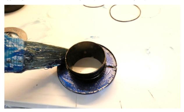
Grease the axial bearing parts with a lot of grease and push them on the inner shell. The grease should make them hold there in this position.
