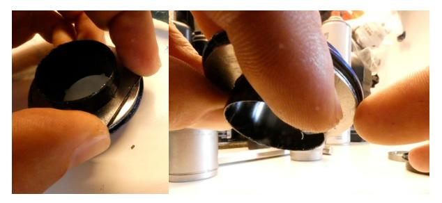
Grease the lower cup on the inside, put in the bearing and put in the o-ring in the groove and lubricate the o-ring a little bit with some oil (doesn't matter which kind of oil).
