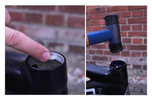
Put spacers, stem and headset on the steerer tube and preload the headset (as tight as possible without influencing a smooth run)
