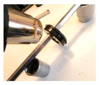
Clean all parts, put in the inner shell in the upper cup, put a small o-ring (the 2 small o-rings have the same size) around the inner shell and grease the inner surface of the upper cup with a salt-water resistant grease (I use Maxima waterproof)
